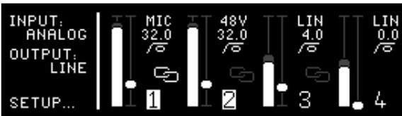
When the analogue inputs are used, a second vertical display is shown for each channel. This is the input gain, and you adjust this by selecting the appropriate channel and turning the encoder.
