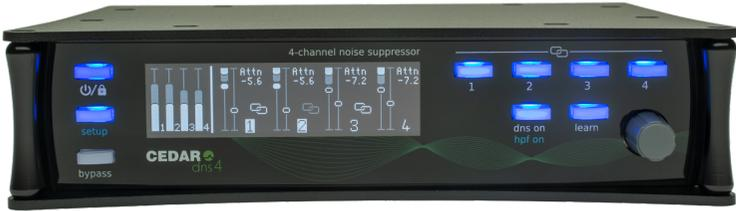
The DNS 4 front panel is divided into three sections: a set of three fixed-function buttons to the left, an OLED screen, plus six context-sensitive buttons and an encoder to the right.
