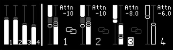
The DNS 4 boots into the Process page and returns to it from any other page after a short timeout. This displays information about all four channels simultaneously.
